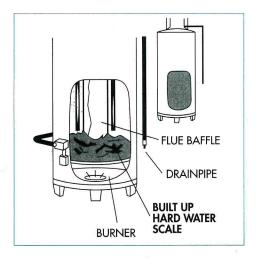
layer of insulation (in the form of scale) between the water and the heat source. Scale acts as an insulator and is a poor conductor of heat.
