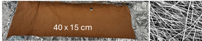
Fig. 2. PTA assisted Nylon-iron oxide nanofiber sheet and its SEM image.
